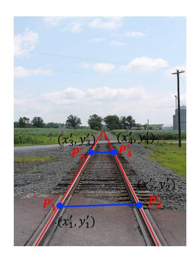
The lengths of two lines  $P_1P_2$  and  $P_3P_4$  in 3D space are equal
