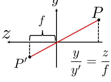
$$P = \begin{bmatrix} x \\ y \\ z \end{bmatrix} \xrightarrow{\text{Nonlinear}} P' = \begin{bmatrix} x' \\ y' \\ y' \end{bmatrix}$$
